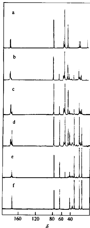
Fig. 1 ^{13}\text{C} -NMR spectra (125MHz) of homopolymer and copolymer samples prepared by group transfer copolymerization of MMA and BA at 22^\circ\text{C} . Spectrum a, PMMA; spectrum b, copolymer with f_M = 0.90 ; spectrum c, copolymer with f_M = 0.74 ; spectrum d, copolymer with f_M = 0.48 ; spectrum e, copolymer with f_M = 0.20 ; spectrum f, PBA
